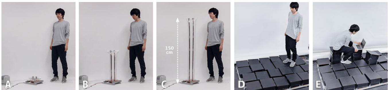
Figure 1: A modular inflatable actuator as a building block for prototyping room-scale shape-changing interfaces. Each actuator can extend from 15 cm to 150 cm (A-C). By constructing these modular blocks, a designer can easily prototype different room-scale shape-changing interfaces, such as a 5 x 5 array of room-scale shape display that a user can sit down and step on (D-E).
