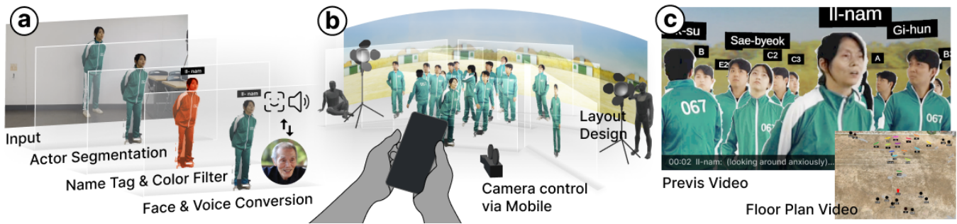
Figure 1: CollageVis composites a film previs through two user interfaces: (a) collage board and (b) virtual stage. The collage board segments actors from the input videos and assigns roles by tagging names, applying color filters, and changing faces and voices. The virtual stage places the video layers, staff, and lighting equipment in 3D space and allows the user to record shots using a mobile as a proxy for the virtual camera. The (c) output of CollageVis includes previs video and floor plan video.
