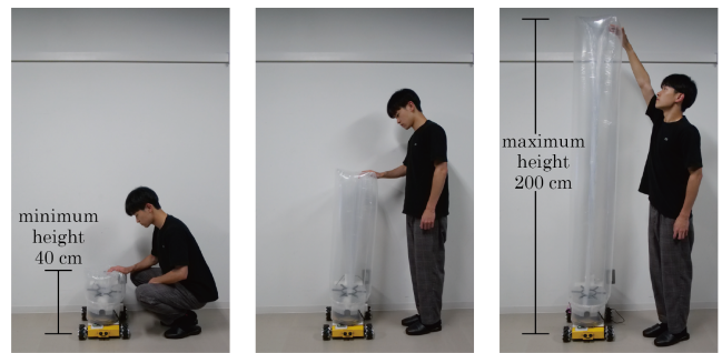
Figure 3: InflatableBots change the height from a minimum of 40 cm to a maximum of 200 cm at 10.4 cm/sec.
