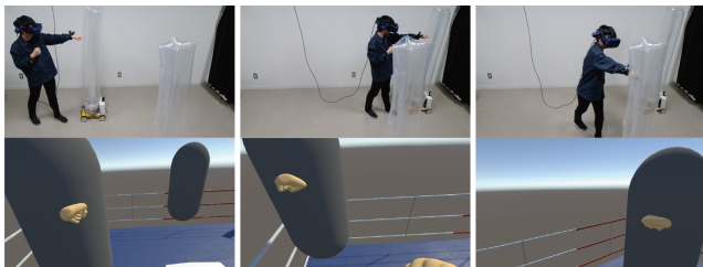
Figure 10: Playing boxing: the user can punch safely by the soft body of InflatableBots.
