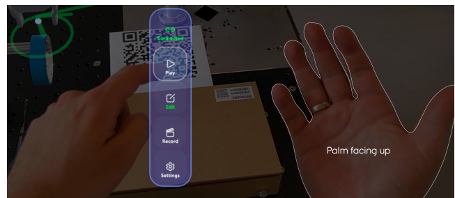
Figure 2: Screenshot of the mode selection interface. The menu is active when the palm of either hand is facing up. The menu can be interacted with using the opposite hand.
