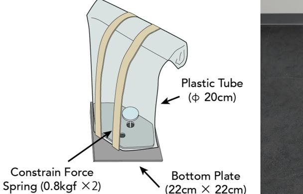
Compact: 15 cm in height Extendable: up to 1.5m with air supply Strong: withstand 10kg object Lightweight: 1.8kg for each unit Large Footprint: 30cm x 30cm Low-cost: \$8 USD for each Modular: reconfigurable (horizontal + vertical)
