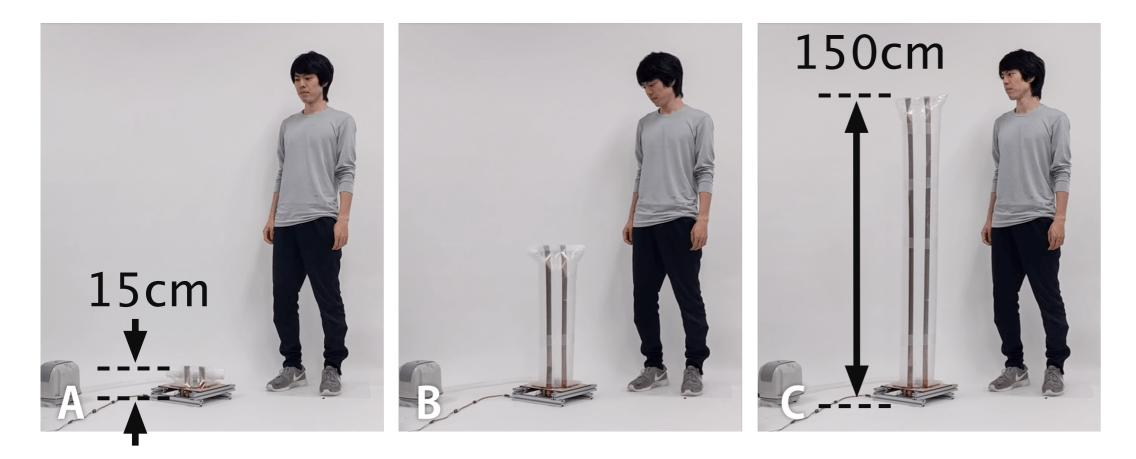
Actuators can extend with air supply and retract with constant force spring
