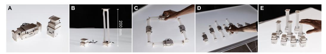
ShapeBots is a prototype system of shapechanging swarm robots, by leveraging highly extendable miniature reel linear actuator (extend from 2cm to 20cm, 3cm x 3 cm size).
