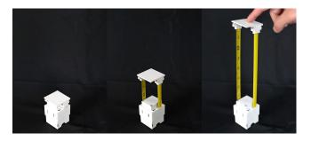
Figure 7: The reel actuator extends the tape at 2.8 cm/sec from a minimum height of 8cm to a maximum height of 32 cm.
