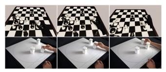
Figure 17: Playing chess: When a user moves a physical piece, the virtual piece moves accordingly and is transmitted to the opponent.
