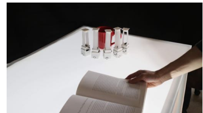
Figure 8: SHAPEBOTS indicates the coffee cup is too hot by creating a vertical fence.
