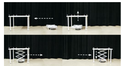
Figure 10: The robot can go beneath a piece of furniture to lift, move and place it.
