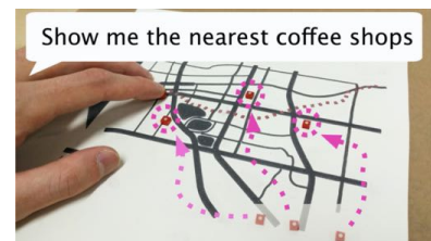
Figure 13: FLUXMARKER actuates magnetic markers to enable the blind user to touch the information.
