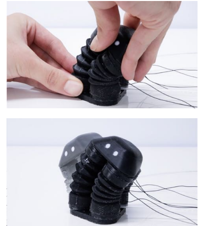
Figure 18: Program soft robots by demonstration. The user can program the simple behavior by physically deforming the soft robot [9].
