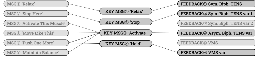
Fig. 6. Summary of the design process: Four key messages were distilled from the initial six messages and remapped to the appropriate electrical stimulation haptic feedback with experts.
