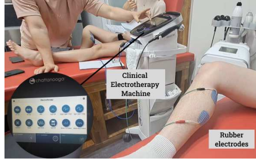
Fig. 4. Electrical stimulation test setup: 2"x2" self-adhesive electrodes were placed at the start and end points of the participant's gastrocnemius muscle. After calibrating the intensity for each person, various clinical electrotherapy settings were applied.
