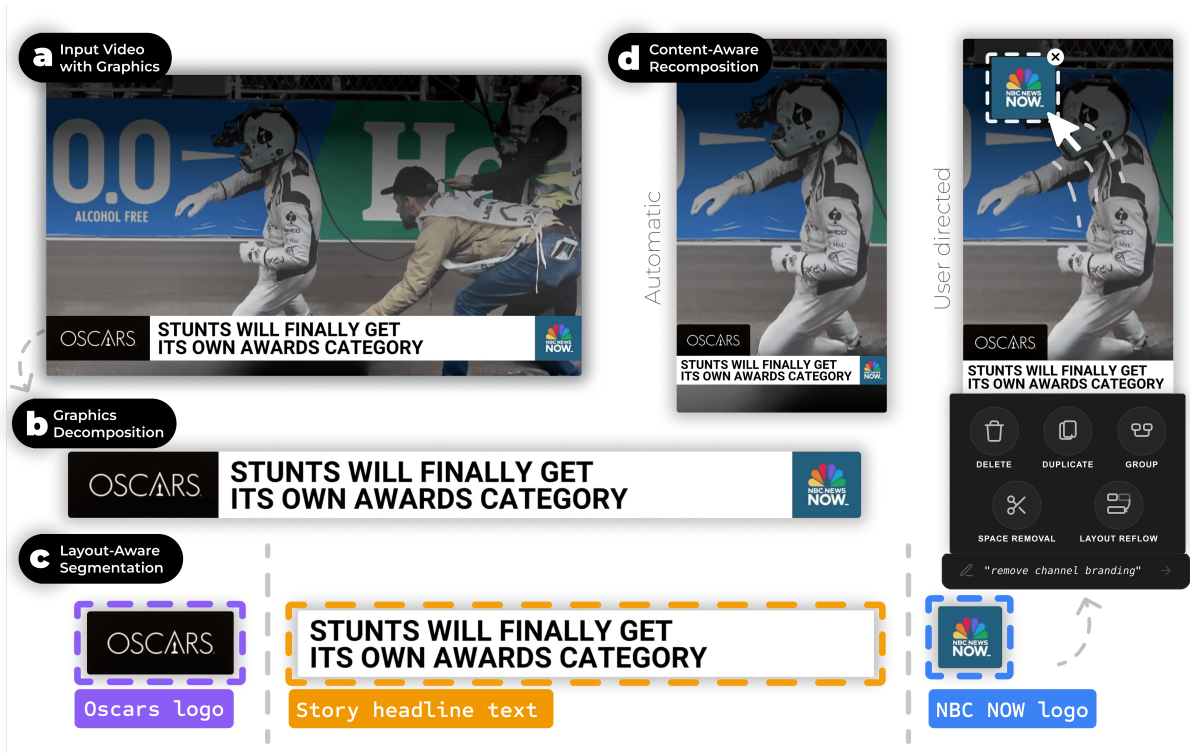
Figure 1: CARVid is a mixed-initiative tool for retargeting on-screen graphics in videos to new aspect ratios while preserving readability and original design intent. Given an input video with embedded graphics (a), CARVid first decomposes the animated graphic from the video (b), then performs layout-aware segmentation on a reference frame to split meaningful elements such as logos, text blocks, and branding (c). Using the recovered structure together with its motion over time, CARVid can automatically recompose the graphic through text-aware scaling, content-aware space removal, and layout reflow, or expose direct editing controls that let users rearrange, group, duplicate, or remove elements (d).
